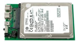
Place your hard drive mechanism onto the bridge card and fully seat the drive onto the connector.
