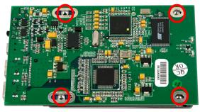
Turn the bridge over and look through the screw holes. Make sure they are fully lined up and insert 4 screws into the hard drive.
