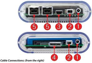
① **DC IN port** - Use an auxiliary power source (not included, and not normally needed) with your OWC Mercury On-The-Go Pro with this port. If you need a power adapter, they are available via separate purchase at:
