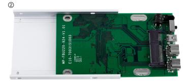
Remove the bridge card from the aluminum heatsink. It just slides in, no screws are holding it in place.
