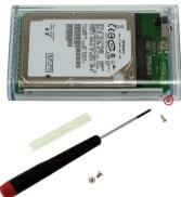
Insert the acrylic endcap, fully sliding it over the bridge card ports.
